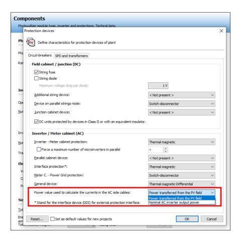
Remember that previously and for old projects, the calculation of the maximum AC power transferred upstream of the inverter was linked to the maximum applicable or applied photovoltaic field.
