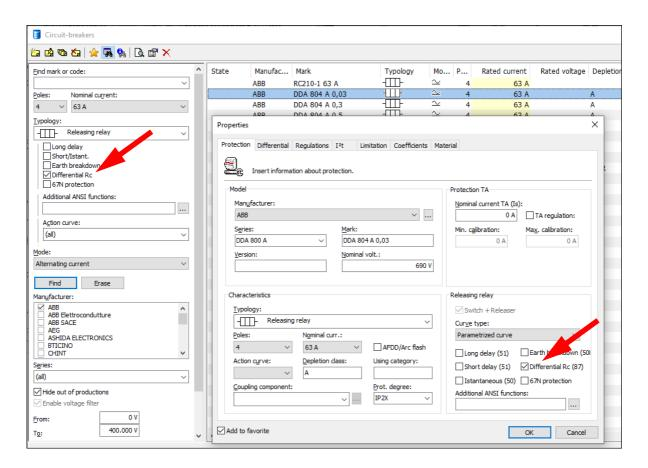
Although in most cases the residual current device is a release relay to be combined with the magnetothermic, the software gives the possibility of assigning a pure differential device as the second element of the MV+D protection as well.
