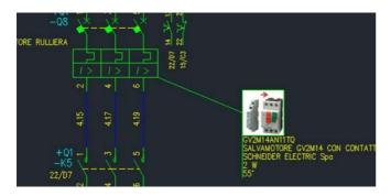
Example of label of a electric plant symbol:
