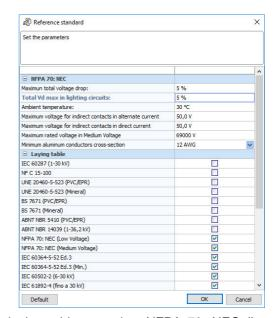
The laying tables, used to NFPA 70: NEC (Low Voltage) and NFPA 70: NEC (medium voltage), manage AWG cables.
