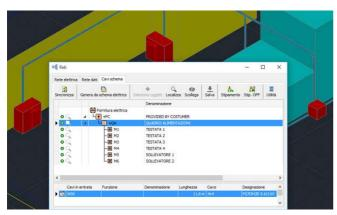
The automatic assignment of the cables identifies for each selected cable, the shortest path of conduit that connects the symbols of component connected by the cable. The cables connecting the two panels, for example, are assigned to the conduits lines that connect the symbols representing the two panels in the drawing. The path search considers the conduits that have the correct destination of use.
