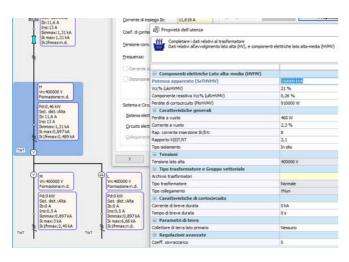
The calculation of networks with three windings transformers follows the standards CEI EN 60909-0, 60909-2 and 60909-4.
