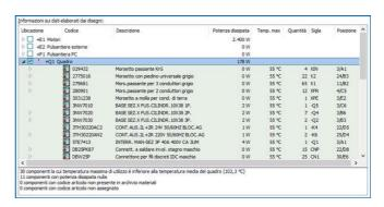
For each component acquired from the circuit diagram, the main grid display the technical data collected from the article database (code, description, power loss, maximum temperature of use), and the data acquired from the circuit diagram (quantity, designation, location in the diagram).
