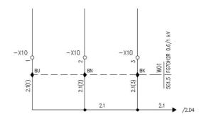
In the example, the terminals -X10 are connected to pins A2 of relays -KF2, -KF3, -KF4 via the same wire 2.1.
