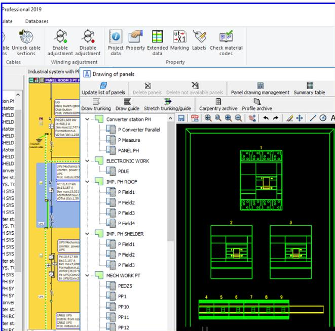
All the necessary tools for the drawing of the panel are available: with the choice in the Carpentry archive of the structure or frame of the cabinet or cabinet, the block of the frame and of the other elements that make up the wardrobe or cabinet is proposed (door , panels, accessories, ...) according to the pre-established compatibility in the database. Also for the drawing of guides and the trunkings, simply select the model from the database and quickly place the pieces on the carpentry.
