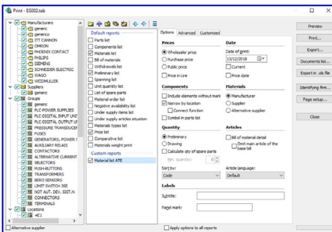
The Parts list is the list of materials in the plant, for which a certain number of spare parts is required. For each item in the bill of materials, the spare parts quantity can be now shown as a percentage. The quantity of spare parts is calculated by applying the percentage parts quantity to the value of the Preliminary quantity or Drawing quantity, based on the option selected in the article database.
