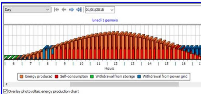
Like the print reports, the daily chart of the energy analysis with precision in the quarter of an hour shows the trend of the energy produced, absorbed and self-consumed, detailing four values for each hour.
