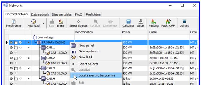
In Network Management, a function has been introduced that facilitates the identification of the electric barycentre of a booth or panel. The Locate electric barycentre command can be started from the context menu and can be executed after having placed booths, panels or loads in the floor plan immediately downstream of the cab to be positioned. An arrow-shaped indicator will indicate the optimal calculated position based on the powers and utilization coefficients involved.
