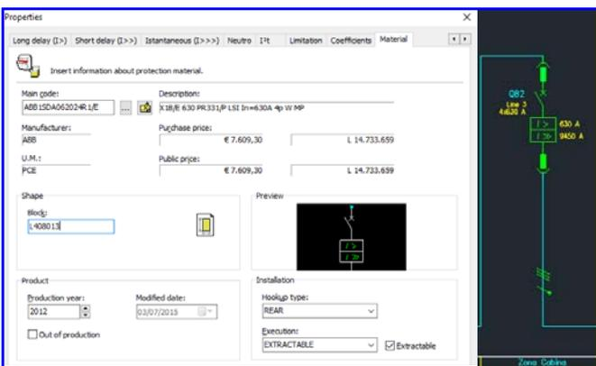
**Recognition of equipment on a single-line diagram for multi-line point-to-point connections**
