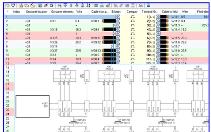
Starting from a selected sheet, the software will make the drawing in the necessary sheets. The diagram shows all the connection levels from the selected terminal block that can be represented in the space available in the sheet. The design order of the terminals of the main terminal board is determined by the index of the terminal board that can be set in Cablo. The terminal block connection diagram is updated automatically using the Update tables function.
