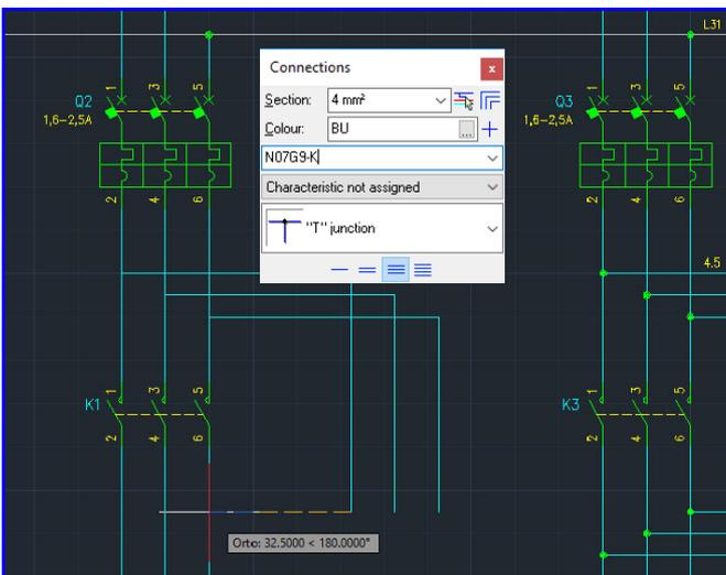
If the number of phases drawn is greater than one, the other lines will automatically identify the corresponding phases on which to connect.
