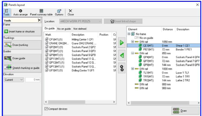
A summary table of the inserted devices can finally be attached to the layout drawing.
