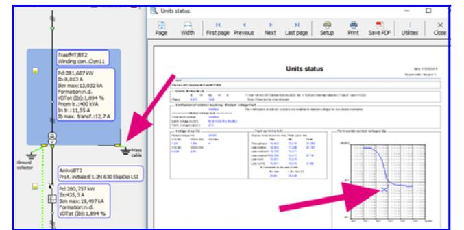
For the verification of the primary side fault of a medium voltage transformer, Ampère calculates the values of the total earth voltage in the user in question given by all the earth fault current that passes on the user's sink, as in the case of cabins powered by overhead lines without a grounded guard line.
